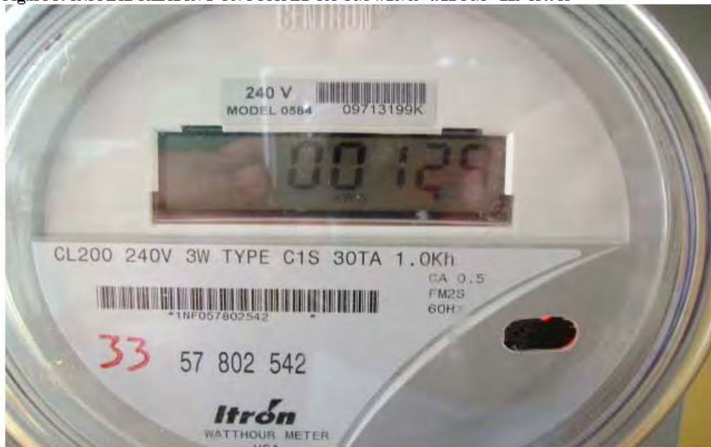
Figure 8: INITIAL READING UNCOATED ROOM 7/10/09 4:11 PM - 129 KWH
