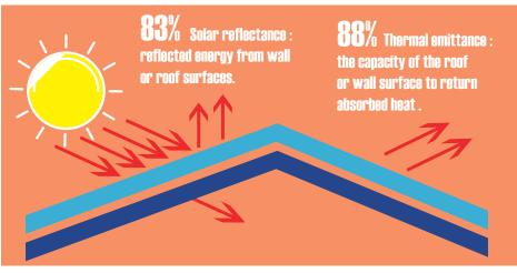
Thermal resistance R = 1,87m2K/W - Thermal transmittance : U = 0,53W/m2K - Solar reflectance index SRI : 104
